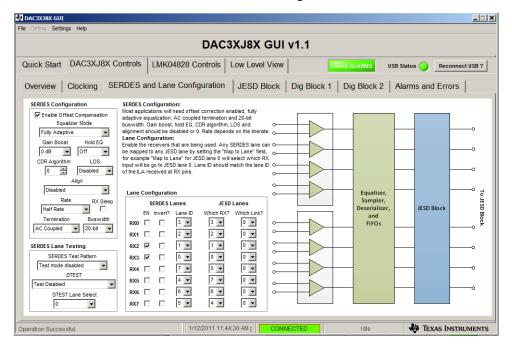
Figure 12. DAC38J8x GUI SERDES Lane Configuration
