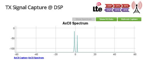
Figure 20. TX Signal Capture at DSP (2-Tone Data Pattern)
