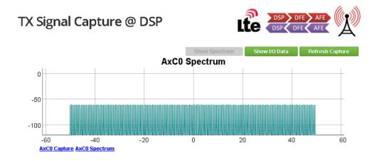
Figure 21. TX Signal Capture at DSP (200-Tone Data Pattern)
