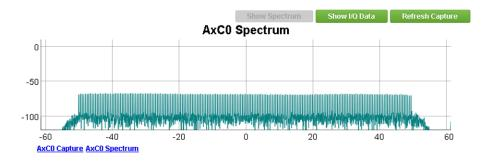
Figure 26. RX Signal Capture at DSP (200-Tone Data Pattern)
