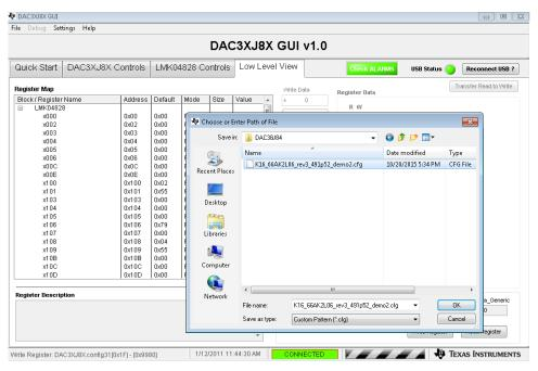
Figure 10. Low Level View to Load Registers
