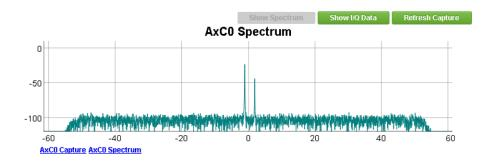
Figure 22. RX Signal Capture at DSP (2-Tone Data Pattern)
