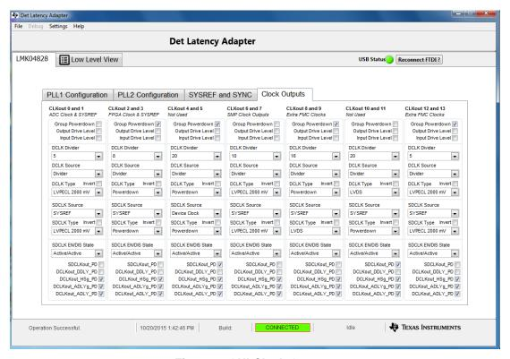
Figure 7. GUI-Clock Outputs
