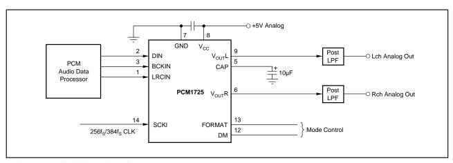
FIGURE 5. Typical Connection Diagram.
