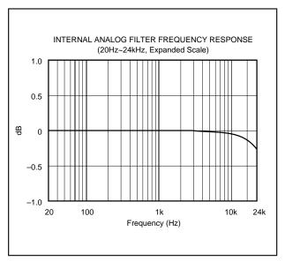
FIGURE 7. Low Pass Filter Frequency Response.
