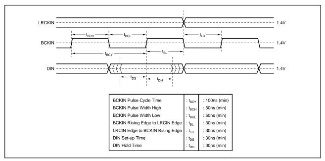
FIGURE 3. Audio Data Input Timing.
