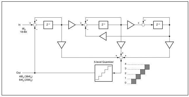
FIGURE 10. 5-Level  $\Delta\Sigma$  Modulator Block Diagram.
