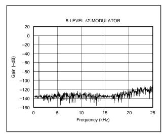
FIGURE 11. Quantization Noise Spectrum.
