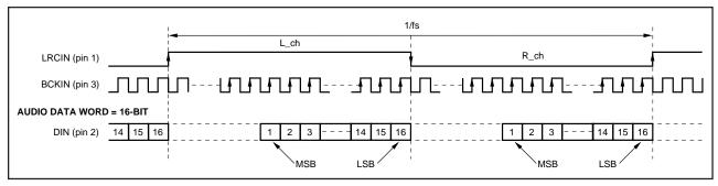
FIGURE 1. "Normal" Data Input Timing.
