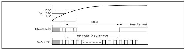
FIGURE 6. Internal Power-On Reset Timing.
