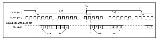
FIGURE 2. "I2S" Data Input Timing.
