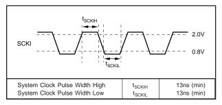
FIGURE 4. System Clock Timing Requirements.
