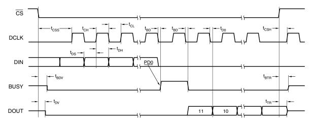
Figure 5. Detailed Timing Diagram
