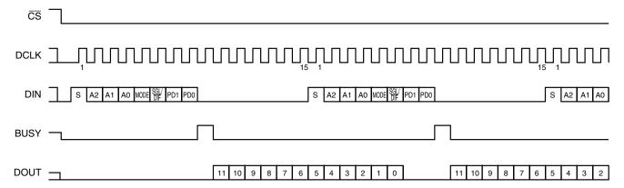
Figure 6. Maximum Conversion Rate, 15 Clock Cycles Per Conversion
