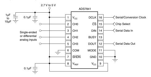
Figure 1. Basic Operation of the ADS7841
