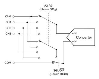
Figure 2. Simplified Diagram of the Analog Input
