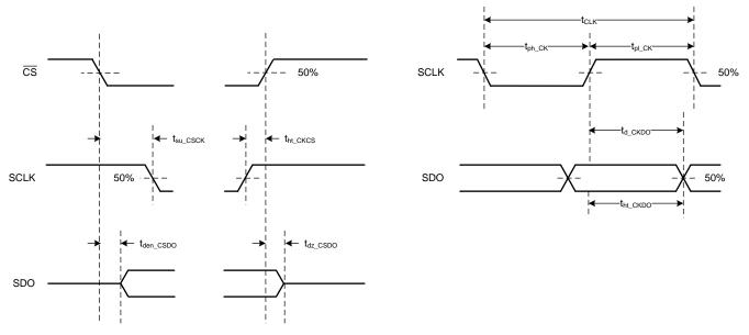
Figure 2. Timing Specifications
