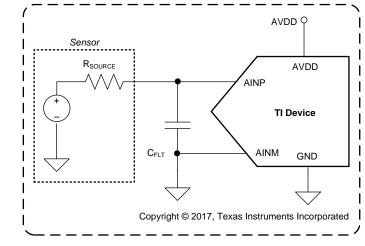
9.2.3 14-Bit, 10-kSPS DAQ Circuit Optimized for DC Sensor Measurements
