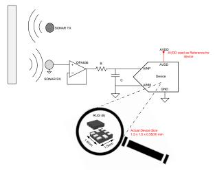
NOTE: The ADS7056 is smaller than a 0805 (2012 metric) SMD component.
