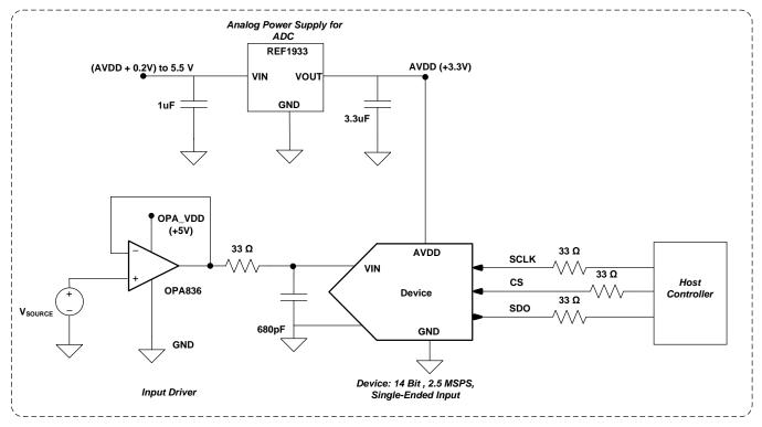
Figure 43. DAQ Circuit: Single-Supply DAQ
