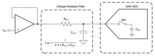
Figure 44. Input Sample-and-Hold Circuit for a Typical SAR ADC
