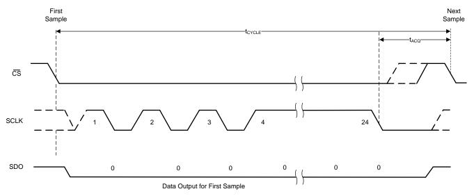
Figure 41. Timing for Offset Calibration on Power-Up
