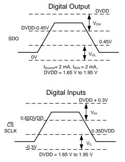
Figure 35. Digital Voltage Levels as per the JESD8-7A Standard
