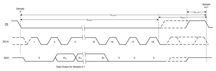
Figure 40. Serial Interface Timing Diagram
