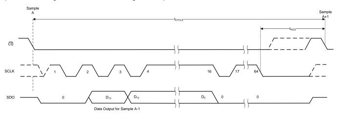
Figure 42. Timing for Offset Calibration During Normal Operation
