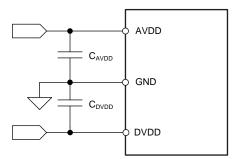
Figure 52. Power-Supply Decoupling
