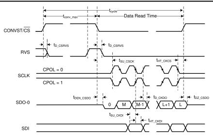
Figure 6-4. Standard SPI Interface Timing Diagram for CPHA = 1
