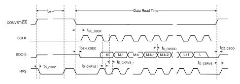
Figure 6-7. multiSPI Source-Synchronous External Clock Serial Interface Timing Diagram
