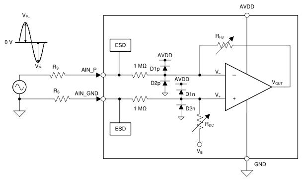
Figure 7-2. Input Overvoltage Protection Circuit Schematic
