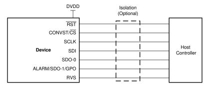
Figure 7-20. All multiSPI Protocols Pin Configuration
