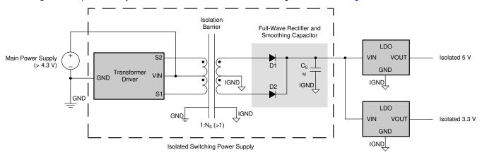
Figure 8-2. Isolated Power-Supply Design
