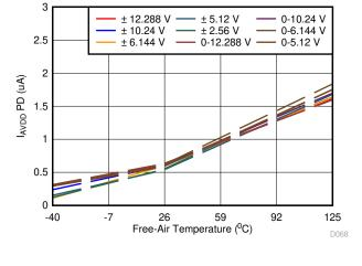
Figure 6-45. AVDD Current vs Temperature (Standby Mode)
