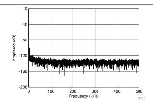
$$\begin{split} f_{SAMPLE} = 1 \text{ Msps, V}_{IN} = \pm 12 \text{ V, f}_{IN} = 1 \text{ kHz, V}_{CM} = 155 \text{ V}_{PP}, \\ \text{SINAD} = 91.5 \text{ dB, THD} = -109 \text{ dB} \end{split}$$
