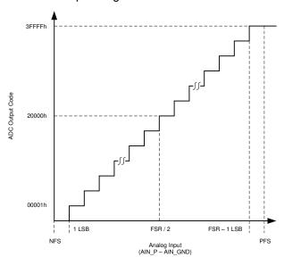
Figure 7-15. Device Transfer Function (Straight-Binary Format)
