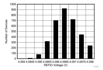
Figure 7-8. Internal Reference Accuracy Histogram at Room Temperature
