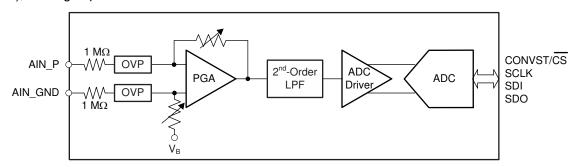
Figure 7-1. Simplified Analog Front-End Circuit Schematic
