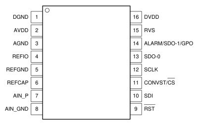
Figure 5-1. PW Package, 16-Pin TSSOP, Top View (Not to Scale)
