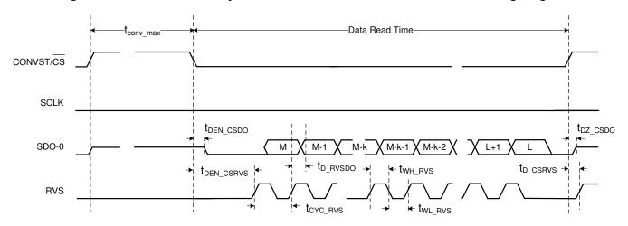
Figure 6-8. multiSPI Source-Synchronous Internal Clock Serial Interface Timing Diagram
