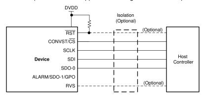
Figure 7-21. Standard SPI Protocol Pin Configuration
