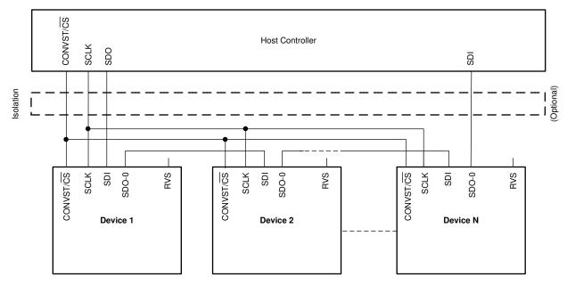
Figure 7-22. Daisy-Chain Connection Schematic
