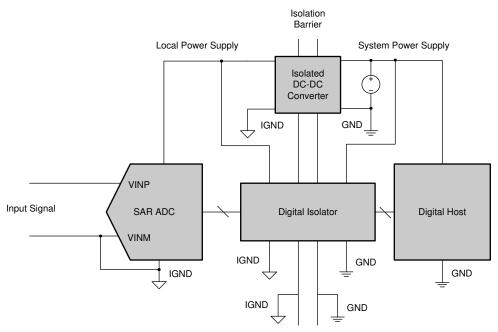
The potential difference between IGND and GND can be as high as the barrier breakdown voltage (often thousands of volts).
