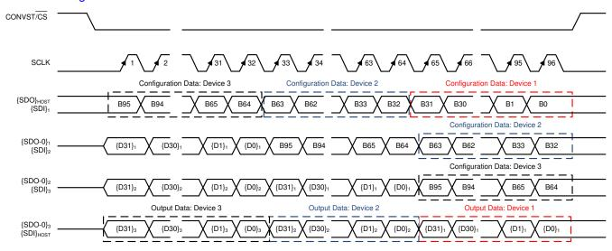
Figure 7-23. Three Devices in Daisy-Chain Mode Timing Diagram
