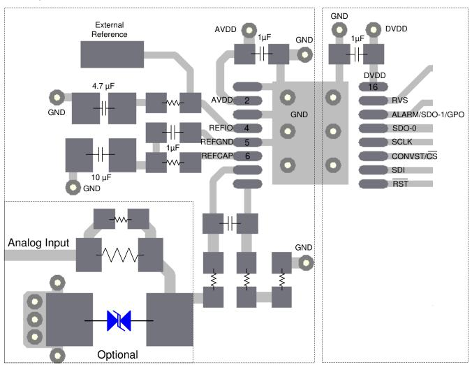
Figure 10-1. Board Layout for the ADS869x
