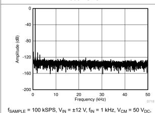
Figure 8-7. FFT Plot With a DC Common-Mode at 100 kSPS
