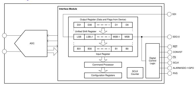
Figure 7-19. Device Interface Module
