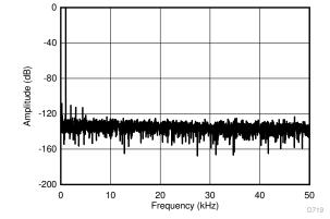
$f_{SAMPLE}$  = 100 kSPS,  $V_{IN}$  =  $\pm$ 12 V,  $f_{IN}$  = 1 kHz,  $V_{CM}$  = 155  $V_{PP}$ , SINAD = 91.4 dB, THD = -109 dB
