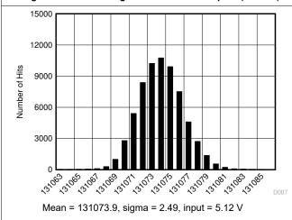
Figure 6-19. DC Histogram for Mid-Scale Inputs (0 V-10.24 V)
