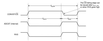
Figure 6-1. Conversion Cycle Timing Diagram
