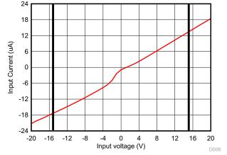
Figure 7-3. I-V Curve for the Input OVP Circuit (AVDD = 5 V)
