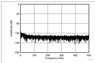
$$\begin{split} f_{SAMPLE} = 1 & \text{MSPS, V}_{IN} = \pm 12 \text{ V, f}_{IN} = 1 \text{ kHz, V}_{CM} = 50 \text{ V}_{DC}, \\ & \text{SINAD} = 92.2 \text{ dB, THD} = -109 \text{ dB} \end{split}$$
