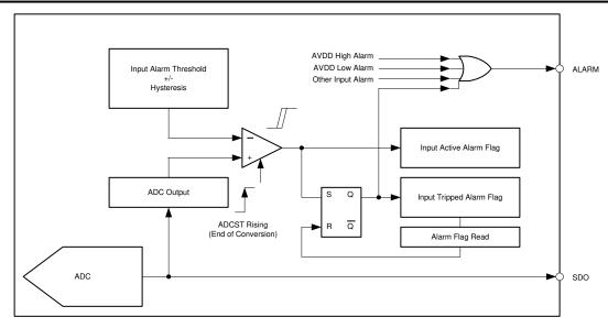
Figure 7-16. Alarm Functionality Schematic
