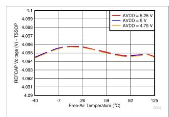
Figure 7-13. Reference Buffer Output (REFCAP)
