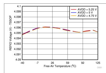
Figure 7-10. REFIO Voltage Variation Across AVDD and Temperature
