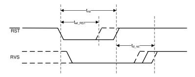
Figure 6-2. Asynchronous Reset Timing Diagram
