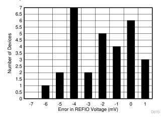
Figure 7-9. Solder Heat Shift Distribution Histogram
