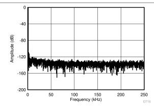
$f_{SAMPLE} = 500 \text{ kSPS}, V_{IN} = \pm 12 \text{ V}, f_{IN} = 1 \text{ kHz}, V_{CM} = 50 \text{ V}_{DC},$ SINAD = 92.3 dB, THD = -109 dB
