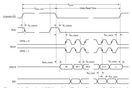
Figure 6-3. Standard SPI Interface Timing Diagram for CPHA = 0
