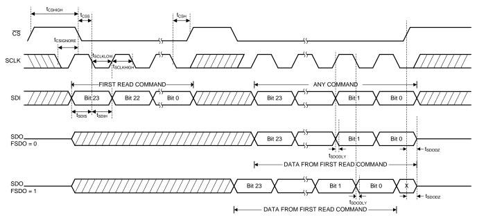
Figure 63. Serial Interface Read Timing Diagram
