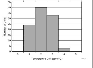
Figure 56. Internal Reference Temperature Drift Histogram
