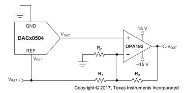
Figure 76. Bipolar Operation Using the DACx0504
