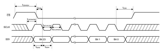
Figure 62. Serial Interface Write Timing Diagram
