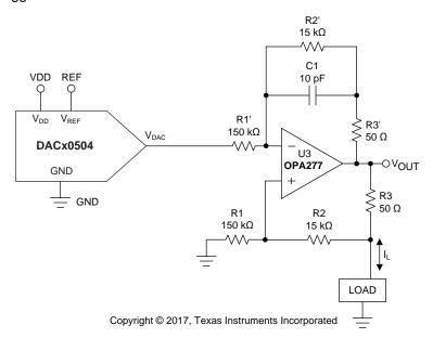
Figure 75. Programmable Bidirectional Current Source Circuit
