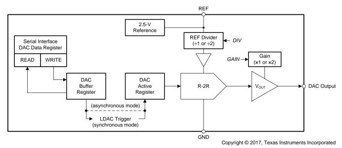
Figure 57. DACx0504 DAC Block Diagram
