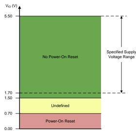
Figure 59. Threshold Levels for V<sub>DD</sub> POR Circuit
