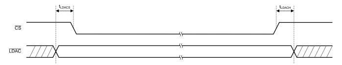
Figure 64. Digital Logic Timing Diagram
