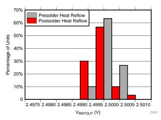
Figure 58. Solder Heat Reflow Reference Voltage Shift
