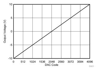
Figure 77. Bipolar Operation
