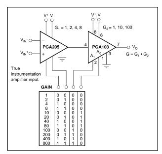
FIGURE 5. Wide Input Voltage Range Amplifer.
