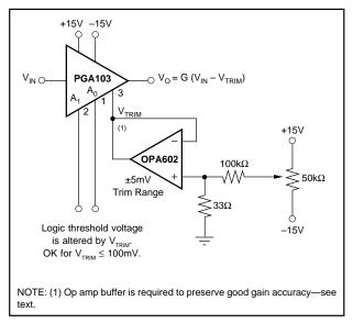
FIGURE 3. Offset Voltage Trim Circuit.
