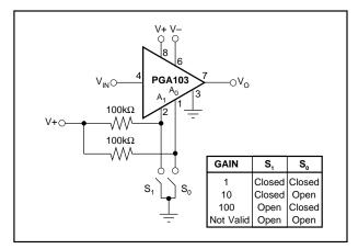
FIGURE 2. Switch or Jumper-Selected Gains.
