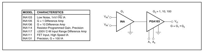
FIGURE 6. Instrumentation Amplifier with Programmable Gain Output Amp.
