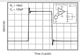
Figure 27. Negative Overload Recovery
