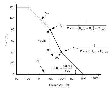
Figure 42. Unity-Gain Amplifier With R<sub>ISO</sub> Compensation
