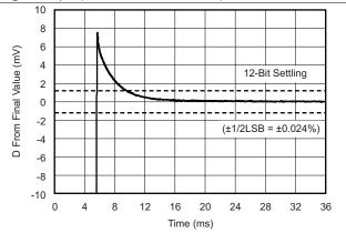
Figure 31. Large-Signal Step Response
