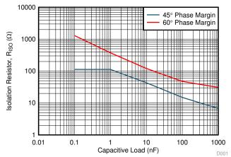
Figure 45. R<sub>ISO</sub> vs C<sub>LOAD</sub>
