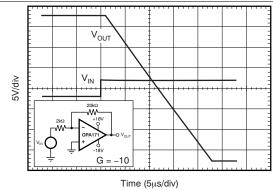
Figure 26. Positive Overload Recovery
