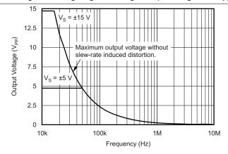
Figure 35. Maximum Output Voltage vs Frequency
