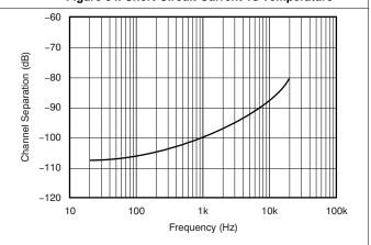
Figure 36. Channel Separation vs Frequency
