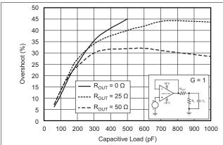
Figure 43. Small-Signal Overshoot vs Capacitive Load (100-mV Output Step)
