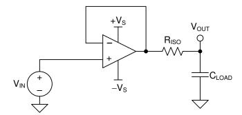
Figure 41. Unity-Gain Buffer With R<sub>ISO</sub> Stability Compensation
