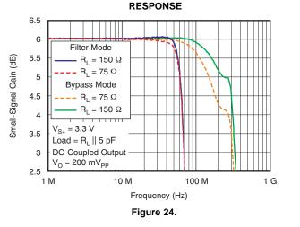
FHD CHANNELS SMALL-SIGNAL GAIN vs FREQUENCY
