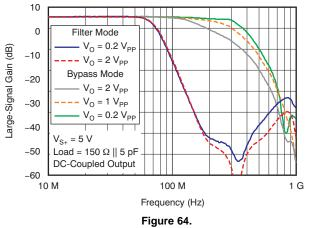
FHD CHANNELS LARGE-SIGNAL GAIN vs FREQUENCY RESPONSE
