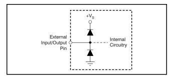
Figure 76. Internal ESD Protection
