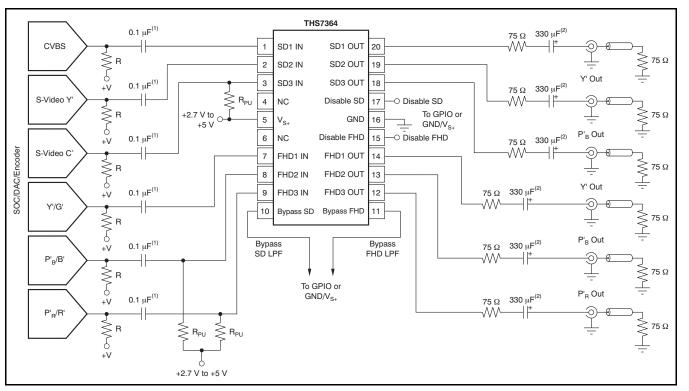
(1) AC-coupled input is shown in this example. DC-coupling is also allowed as long as the DAC output voltage is within the allowable linear input and output voltage range of the THS7364. To apply dc-coupling, remove the 0.1- $\mu$ F input capacitors and the R<sub>PU</sub> pull-up resistors along with connecting the DAC termination resistors (R) to ground.
