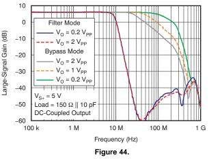
SD CHANNELS LARGE-SIGNAL GAIN vs FREQUENCY RESPONSE
