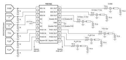
Figure 1. Single-Supply, DC-Input/DC-Output Coupled Video Line Driver
