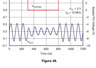
SD CHANNELS BYPASS MODE RESPONSE vs TIME
