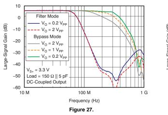
FHD CHANNELS LARGE-SIGNAL GAIN vs FREQUENCY RESPONSE
