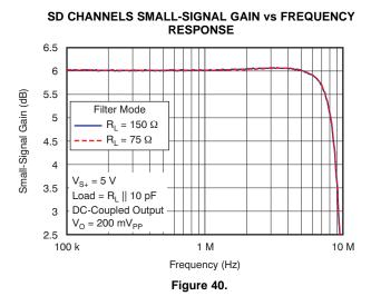
SD CHANNELS SMALL-SIGNAL GAIN vs FREQUENCY RESPONSE
