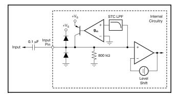
Figure 79. Equivalent AC Sync-Tip-Clamp Input Circuit
