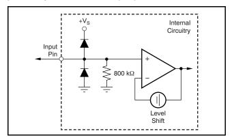
Figure 78. Equivalent DC Input Mode Circuit
