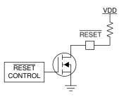
Figure 8-6. Open-Drain RESET Configuration
