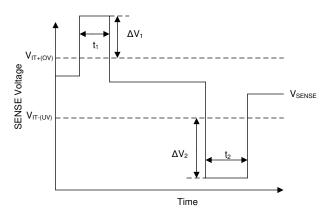
Figure 8-4. Overdrive Voltage on the SENSE Pin
