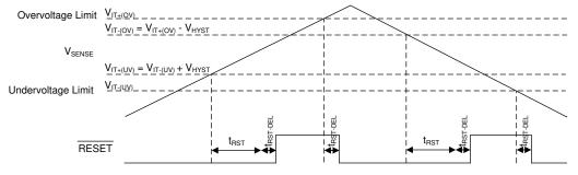
Figure 7-3. Window Comparator Timing Diagram
