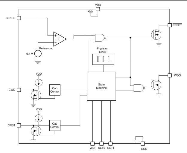
Figure 7-2. Adjustable Version Block Diagram
