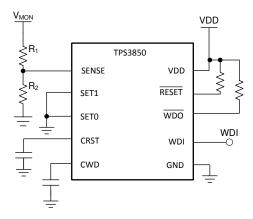
Figure 7-4. Adjustable Voltage Monitor
