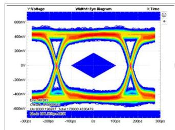
Figure 19. Eye Pattern Error Histogram: 3.0 Gbps With No Device
