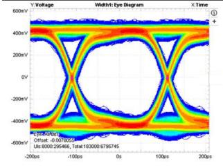
Figure 23. Eye Pattern Error Histogram: 4.5 Gbps With No Device
