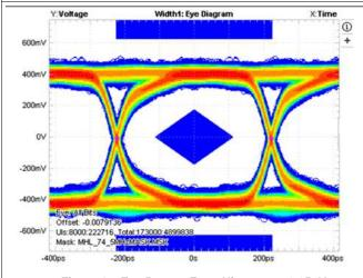
Figure 17. Eye Pattern Error Histogram: 2.25 Gbps With TS3USB3031 (Added Jitter = 5.04 ps)
