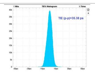
Figure 18. Time Interval Error Histogram: 2.25 Gbps With TS3USB3031 (Added Jitter = 5.04 ps)
