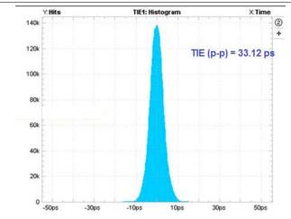
Figure 22. Time Interval Error Histogram: 3.0 Gbps With TS3USB3031 (Added Jitter = 2.57 ps)
