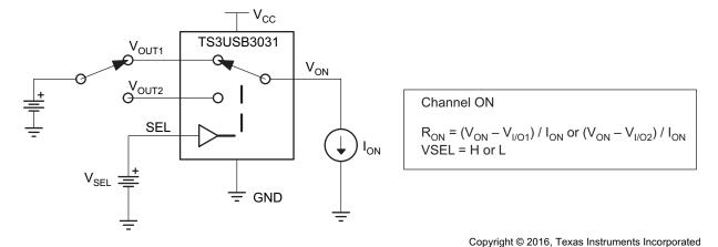
Figure 9. ON-State Resistance (R<sub>ON</sub>)
