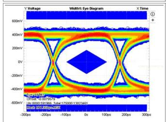
Figure 21. Eye Pattern Error Histogram: 3.0 Gbps With TS3USB3031 (Added Jitter = 2.57 ps)
