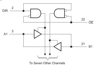
Figure 7-1. Logic Diagram (Positive Logic)
