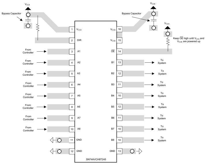
Figure 8-3. SN74AVCH8T245 Layout Example
