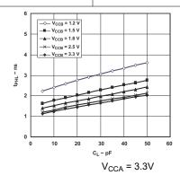
Figure 5-9. Typical Propagation Delay (A to B) vs Load Capacitance
