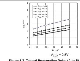
Figure 5-7. Typical Propagation Delay (A to B) vs Load Capacitance
