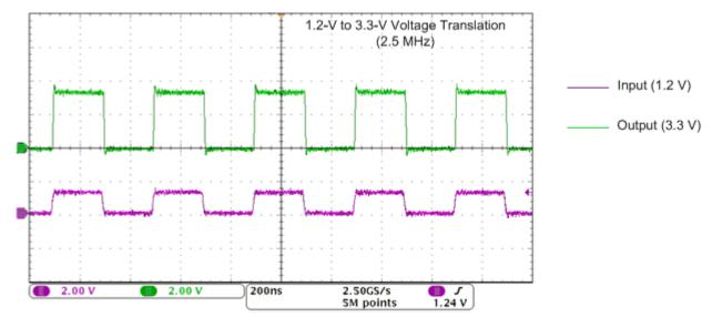
Figure 9-2. Translation Up (1.2V to 3.3V) at 2.5MHz
