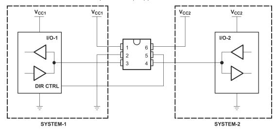
Figure 9-3. Bidirectional Logic Level-Shifting Application Diagram
