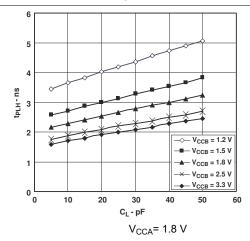
Figure 6-5. Typical Propagation Delay (A to B) vs Load Capacitance
