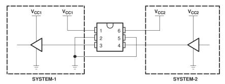
Figure 9-1. Unidirectional Logic Level-Shifting Application Diagram
