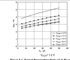
Figure 6-1. Typical Propagation Delay (A to B) vs Load Capacitance
