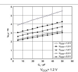
Figure 6-2. Typical Propagation Delay (A to B) vs Load Capacitance
