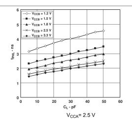
Figure 6-8. Typical Propagation Delay (A to B) vs Load Capacitance
