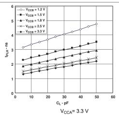
Figure 6-9. Typical Propagation Delay (A to B) vs Load Capacitance
