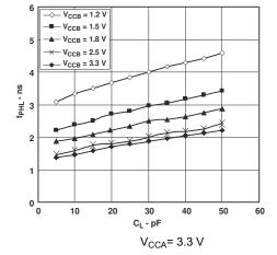
Figure 6-10. Typical Propagation Delay (A to B) vs Load Capacitance
