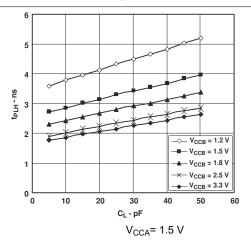
Figure 6-3. Typical Propagation Delay (A to B) vs Load Capacitance
