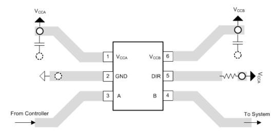
Figure 11-1. PCB Layout Example
