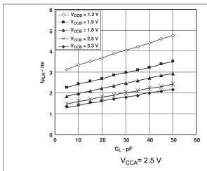
Figure 6-7. Typical Propagation Delay (A to B) vs Load Capacitance
