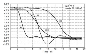
Figure 8-2. Switching Characteristics Comparison
