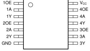
Figure 4-1. BQA Package, 14-Pin WQFN (Top View)
