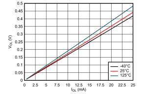
Figure 5-1. Output Voltage vs Current in HIGH State; 5-V Supply | Figure 5-2. Output Voltage vs Current in LOW State; 5-V Supply
