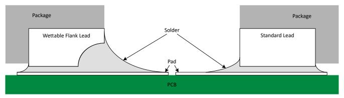
Figure 7-3. Simplified Cutaway View of Wettable-Flank QFN Package and Standard QFN Package After Soldering
