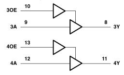
Logic Diagram (Positive Logic)
