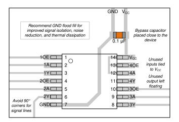
Figure 8-3. Example Layout for the SN74AHCT126-Q1
