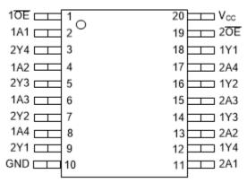
Figure 5-1. DW or PW Package (Top View)
