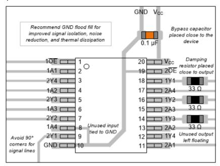
Figure 9-1. Layout Diagram
