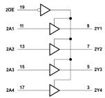
Figure 3-1. Logic Diagram (Positive Logic)
