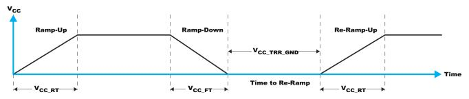
Figure 10-1.  $V_{CC}$  is Lowered Below 0.2 V or 0 V and Then Ramped up to  $V_{CC}$
