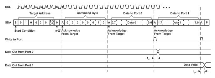
Figure 8-8. Write to Output Port Register
