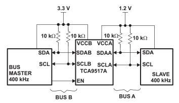
Figure 7. Typical Application Schematic
