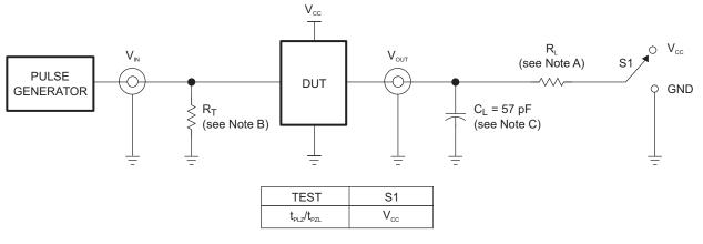
TEST CIRCUIT FOR OPEN-DRAIN OUTPUT
