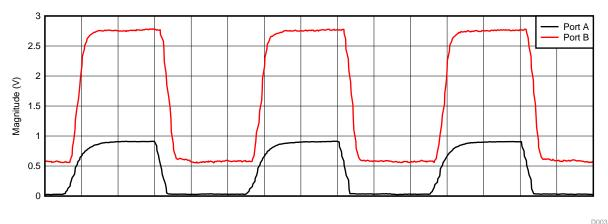
Figure 12. Voltage Translation at 400 kHz,  $V_{CCA} = 0.9 V$ ,  $V_{CCB} = 2.7 V$
