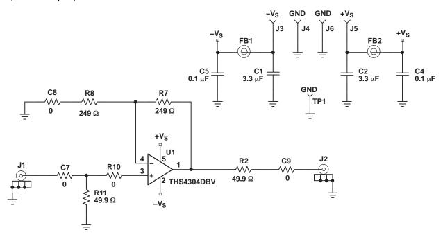
Figure 42. Non-Inverting Gain With Split Power Supply
