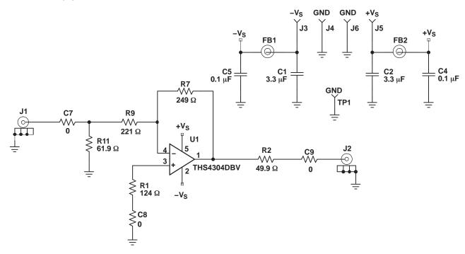
Figure 43. Inverting Gain With Split Power Supply
