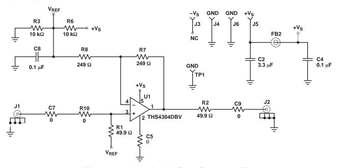
Figure 44. Non-Inverting 5-V Single-Supply Amplifier
