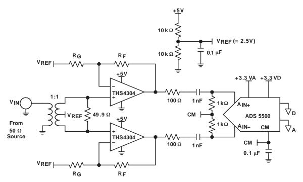
Figure 45. Differential ADC Drive Amplifier Circuit
