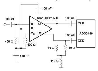
Figure 41. Differential Clock Using PECL Logic
