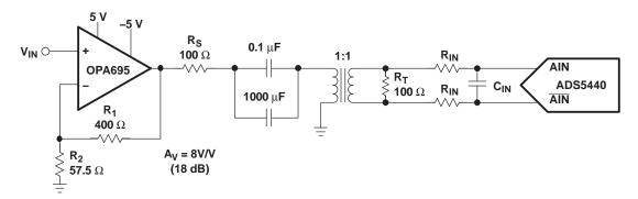
Figure 37. Using the OPA695 With the ADS5440
