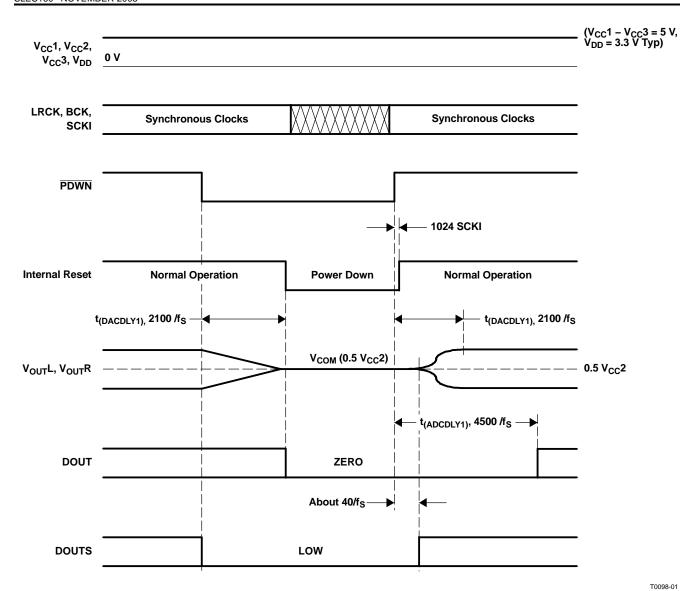
Figure 45. DAC Output and ADC Output for External Reset (PDWN Pin)
