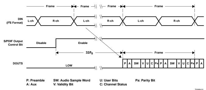
Figure 51. S/PDIF Output Timing
