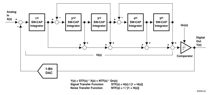
Figure 39. Block Diagram of Fifth-Order Delta-Sigma Modulator
