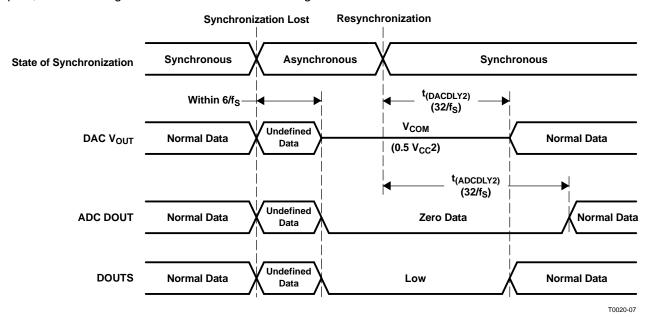
Figure 48. DAC Output and ADC Output for Loss of Synchronization
