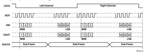
Figure 46. Audio Data Input/Output Format
