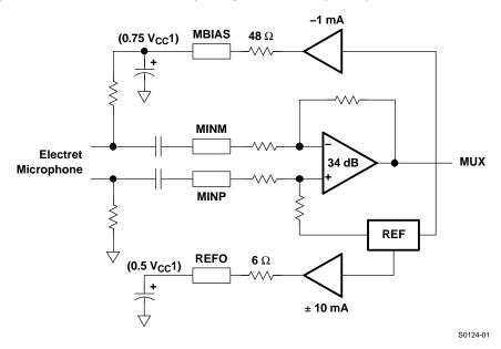
Figure 49. Microphone Amplifier, Microphone Bias Generator, and Reference Output
