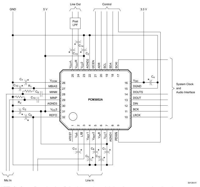
NOTE:  $C_1$ -  $C_4$ : 0.1- $\mu$ F ceramic and 10- $\mu$ F electrolytic capacitors typical, depending on power supply quality and pattern layout.
