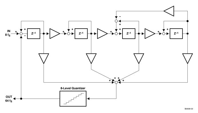
Figure 40. 8-Level Delta-Sigma Modulator Block Diagram
