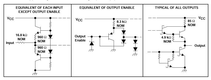
Figure 7-1. Schematics of Inputs and Outputs
