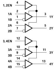
**Logic Diagram (Positive Logic)**
