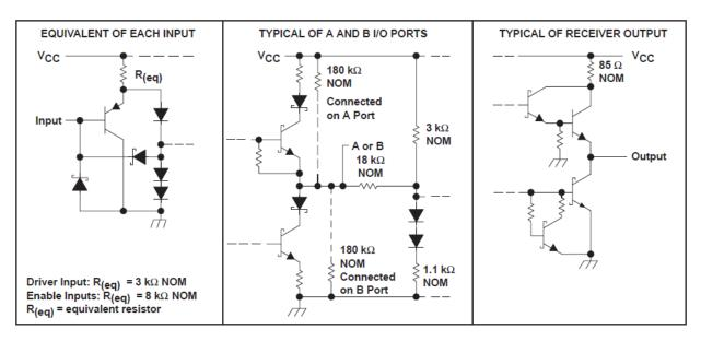
Figure 8-1. Schematics of Inputs and Outputs
