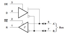
**Logic Diagram (Positive Logic)**
