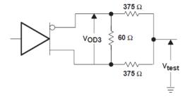
Figure 7-2. Driver V<sub>OD3</sub> Test Circuit
