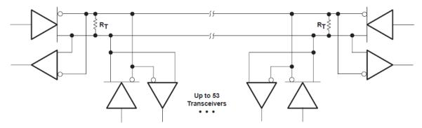
A. The line should terminate at both ends in its characteristic impedance (R<sub>T</sub> = Z<sub>O</sub>). Stub lengths off the main line should be kept as short as possible.
