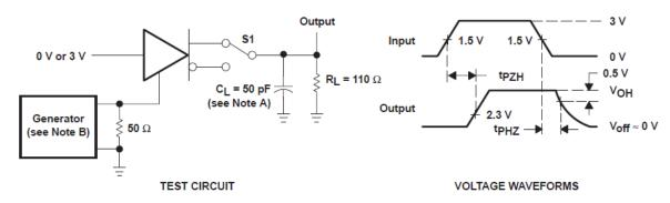
A. C<sub>L</sub> includes probe and jig capacitance.
