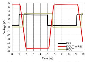
Figure 9-2. 250 kbps Driver to Receiver Loopback Timing Waveform, V<sub>CC</sub>= 3.3 V
