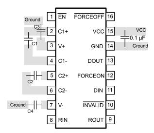
Figure 10-1. Layout Diagram
