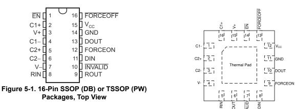
Figure 5-2. 16-pin VQFN (RGT) Package, Top View
