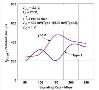
Figure 5-8. Added Receiver Peak-to-Peak Jitter vs Signaling Rate
