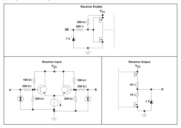
Figure 7-1. Equivalent Input and Output Schematic Diagrams
