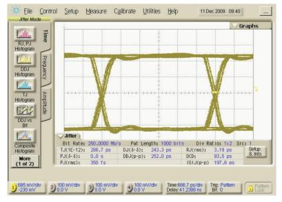
Figure 5-11. Output ( $V_{CC}$  = 3.3V,  $V_{ID}$  = 400mV) 250Mbps 2<sup>15</sup>–1PRBS, Receiver Type 1
