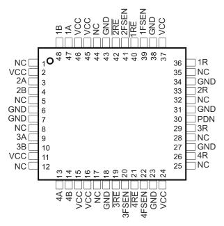
Figure 4-1. RGZ Package (Top View)
