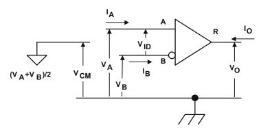
Figure 6-1. Receiver Voltage and Current Definitions
