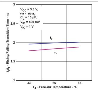
Figure 5-4. Receiver (Type-1) Transition Time vs Free-Air Temperature
