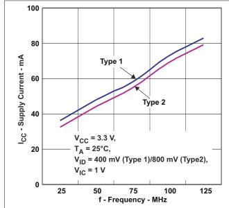
Figure 5-1. Supply Current vs Frequency
