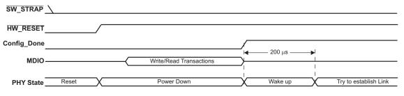
Figure 3-5. TLK111 SW Strap Timing Diagram
