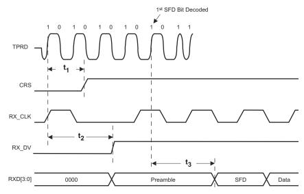
Figure 9-15. 10Base-T Receive Timing (Start of Packet)
