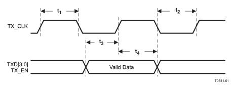
Figure 9-4. 100Mb/s MII Transmit Timing
