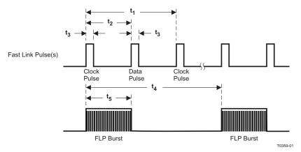
Figure 9-19. Auto-Negotiation Fast Link Pulse (FLP) Timing
