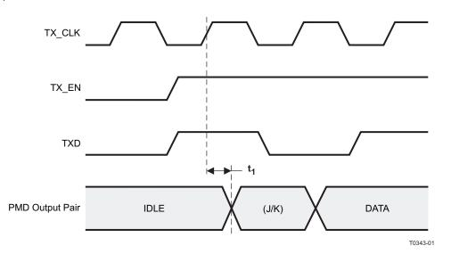
Figure 9-6. 100Base-TX Transmit Packet Latency Timing
