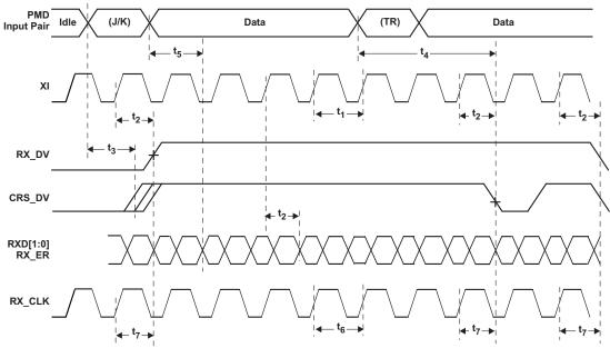
Figure 9-24. RMII Receive Timing
