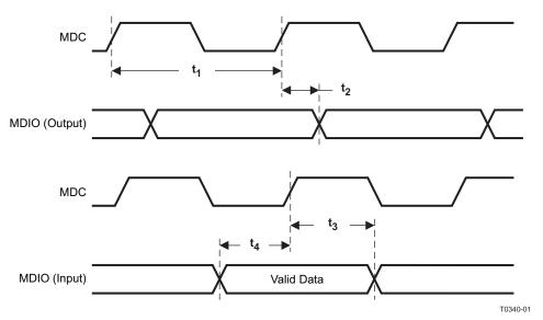
Figure 9-3. MII Serial Management Timing
