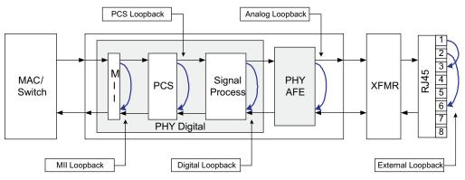
Figure 3-7. Block Diagram, Near-End Loopback Mode
