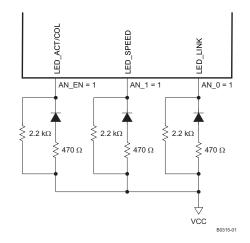
Figure 3-6. AN Pin Configuration and LED Loading Example
