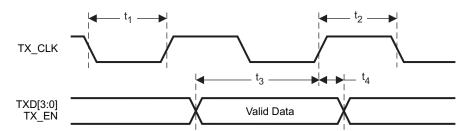
Figure 9-11. 10Mbs MII Transmit Timing
