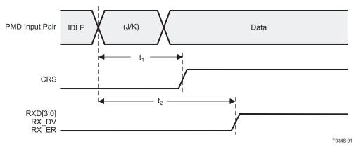
Figure 9-9. 100Base-TX Receive Packet Latency Timing
