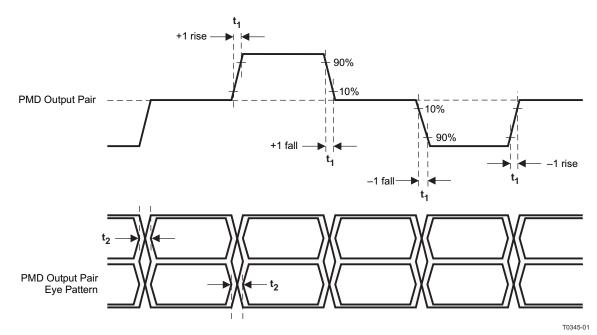
Figure 9-8. 100Base-TX Transmit Timing (t<sub>R/F</sub> and Jitter)
