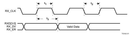
Figure 9-5. 100Mb/s MII Receive Timing
