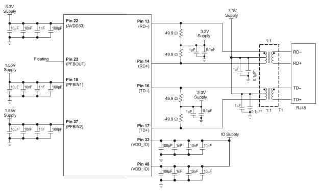
Figure 3-2. Power Connections for Dual Supply Operation
