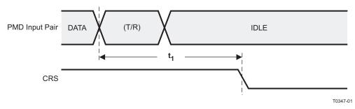
Figure 9-10. 100Base-TX Receive Packet Deassertion Timing
