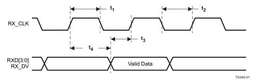
Figure 9-12. 10Mb/s MII Receive Timing
