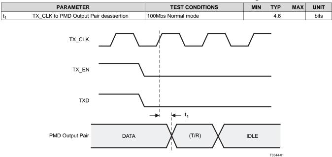
Table 9-7. 100Base-TX Transmit Packet Deassertion Timing
