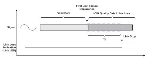
Figure 5-3. TLK111 Link Loss Mechanism
