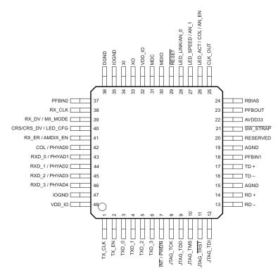
Figure 2-1. TLK111 PIN DIAGRAM, TOP VIEW
