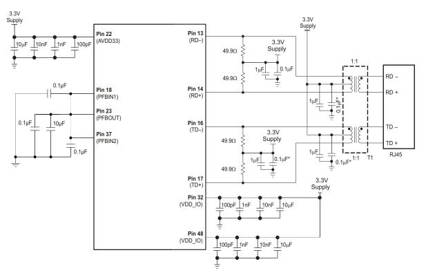
Figure 3-1. Power Connections for Single Supply Operation
