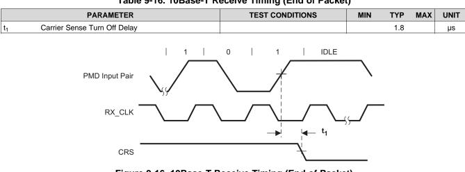
Table 9-16. 10Base-T Receive Timing (End of Packet)
