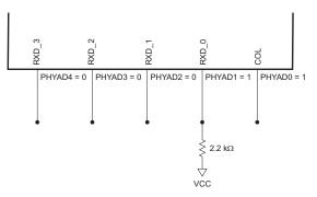
Figure 3-3. PHYAD Configuration Example
