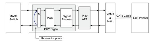
Figure 3-8. Block Diagram, Far-End Loopback Mode
