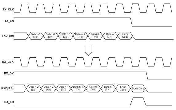
Figure 5-2. Transmit Code Error Forwarding Diagram
