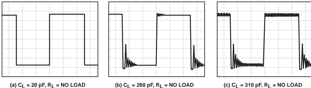
Figure 44. Effect of Capacitive Loads in Low-Bias Mode
