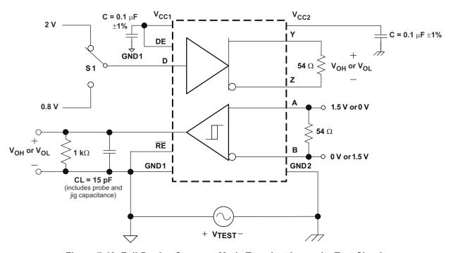
Figure 7-13. Full-Duplex Common-Mode Transient Immunity Test Circuit
