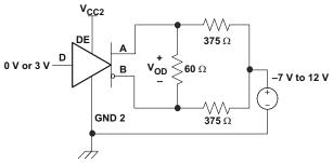
Figure 7-2. Driver V<sub>OD</sub> With Common-Mode Loading Test Circuit
