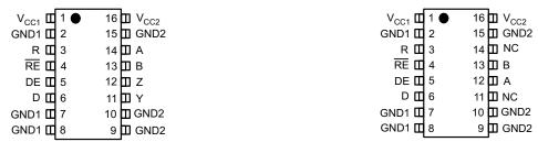
Figure 5-1. ISO3080 and ISO3086 DW Package 16-Pin SOIC Top View Fin SOIC Top View Fin SOIC Top View
