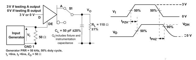
Figure 7-5. Driver High-Level Output Enable and Disable Time Test Circuit and Voltage Waveforms
