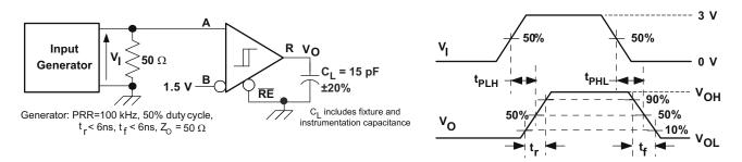
Figure 7-8. Receiver Switching Test Circuit and Waveforms
