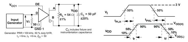
Figure 7-4. Driver Switching Test Circuit and Voltage Waveforms
