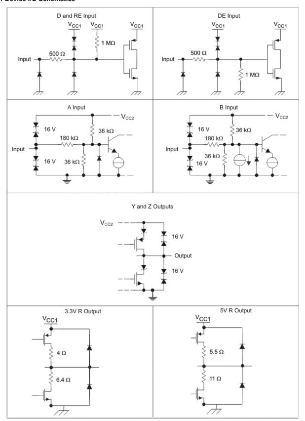
Figure 8-3. Device I/O Schematics
