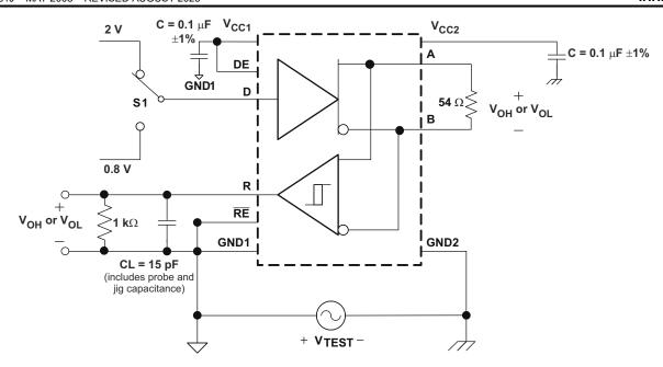
Figure 7-12. Half-Duplex Common-Mode Transient Immunity Test Circuit
