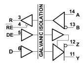
Figure 8-1. ISO3080, IOS3086 Functional Diagram
