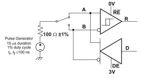
Note: This test is conducted to test survivability only. Data stability at the R output is not specified.
