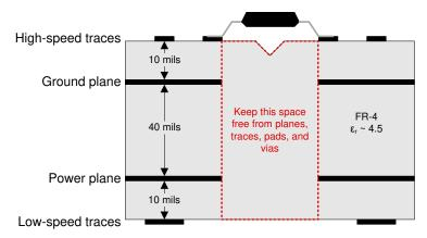
Figure 11-1. Recommended Layer Stack
