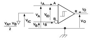
Figure 7-7. Receiver Voltage and Current Definitions
