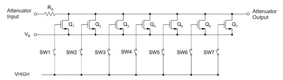
Figure 64. Simplified Voltage-Controlled Attenuator (Digital Structure)
