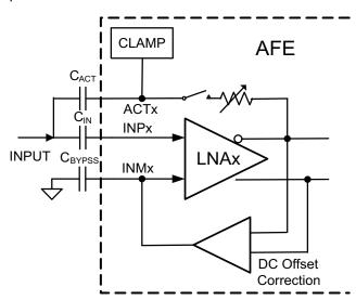
Figure 62. AFE5809 LNA With DC Offset Correction Circuit
