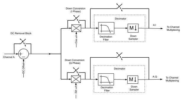
Figure 75. Digital Demodulator Block
