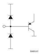
Figure 78. Equivalent Circuits of V<sub>CNTLP/M</sub>
