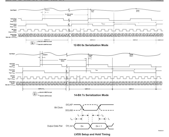
Figure 1. LVDS Timing Diagrams
