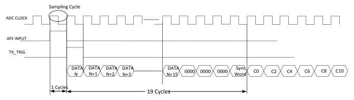
Figure 95. Measured Latency Timing When M = 2
