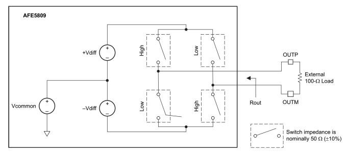
Figure 81. Equivalent Circuits of LVDS Outputs
