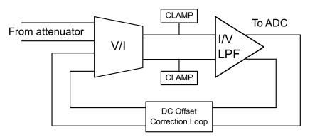
Figure 65. Simplified Block Diagram of PGA
