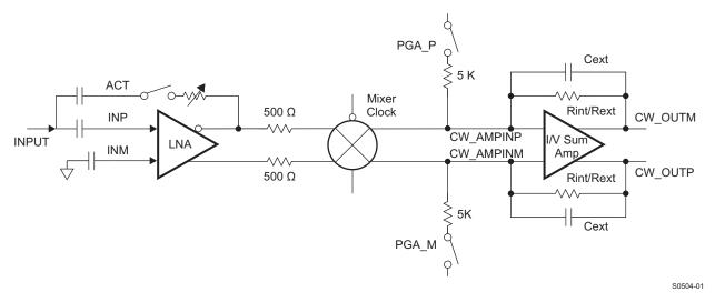
Figure 112. AFE5809 PGA Test Mode
