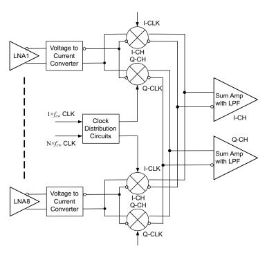
Figure 66. Simplified Block Diagram of CW Path
