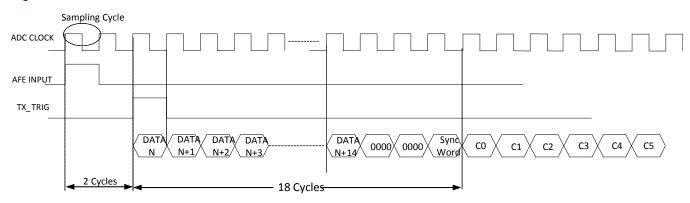
Figure 94. Measured Latency Timing When M = 1
