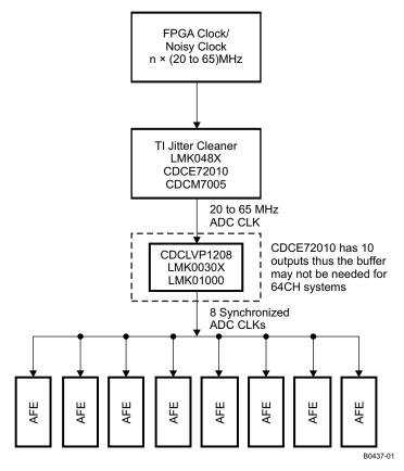
Figure 109. ADC Clock Distribution Network
