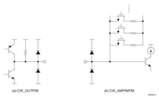
Figure 80. Equivalent Circuits of CW Summing Amplifier Inputs and Outputs
