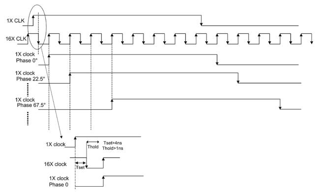
Figure 70. 1x and 16x CW Clock Timing
