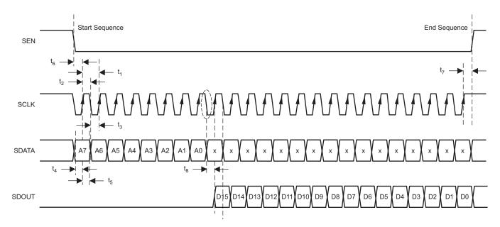
Figure 84. Serial Interface Register Read
