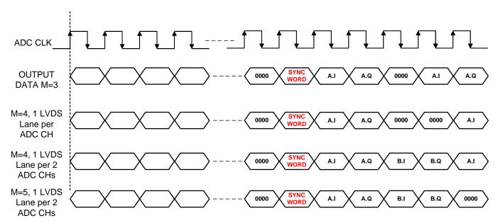
Figure 87. Output Data Format at M = 3~5
