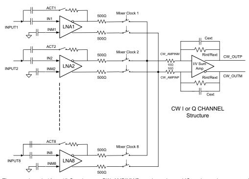
Note: The approximately 10- to 15- $\Omega$  resistors at CW\_AMPINM/P are due to internal IC routing and can create slight attenuation.
