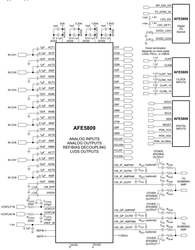
Figure 98. Application Circuit With Digital Demodulator
