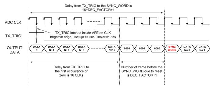
Figure 92. Sync Word Generation With Respect to TX\_TRIG when DC\_REMOVAL\_BYPASS 10[0] = 0
