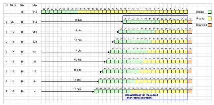
Figure 88. Shifted Output When DEC\_SHIFT\_SCALE=0
