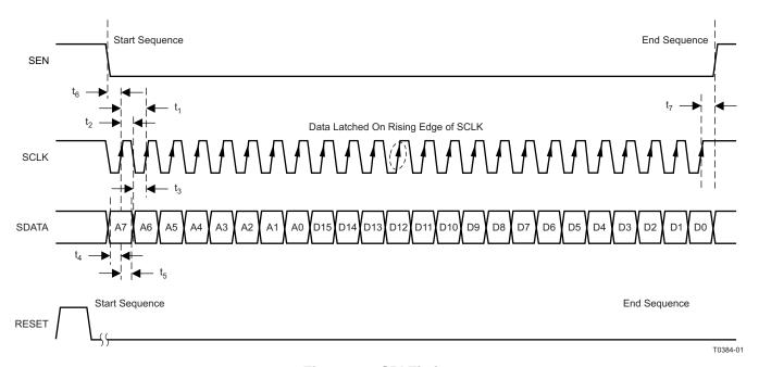
Figure 83. SPI Timing
