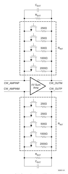
Figure 104. CW Summing Amplifier Block Diagram
