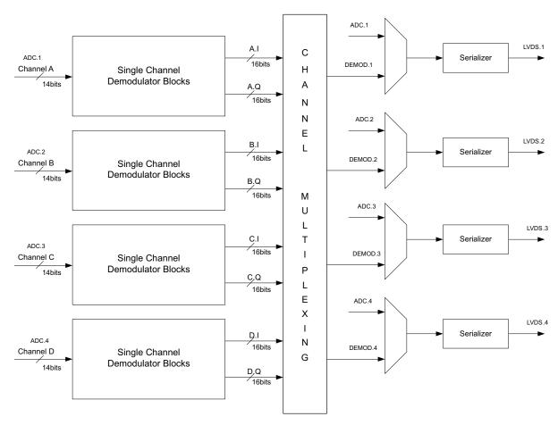
Figure 76. Channel Multiplexing
