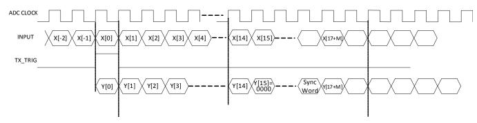
Figure 97. Typical Timing Expression Among ADC CLK, Input, TX\_TRIG, and Output
