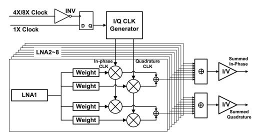
Figure 71.  $8 \times f_{cw}$  and  $4 \times f_{cw}$  Block Diagram
