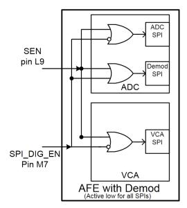
Figure 82. SPI Interface in the AFE5809 Device
