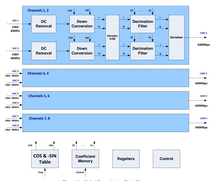
Figure 61. Digital Demodulator Block Diagram
