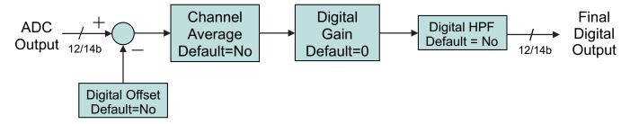
Figure 86. ADC Digital Block Diagram
