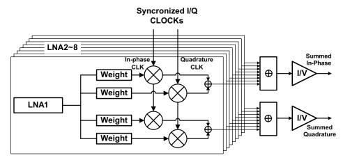
Figure 73. Block Diagram of 1 x  $f_{cw}$  mode
