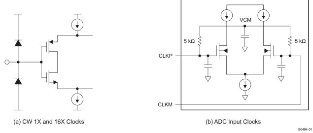
Figure 79. Equivalent Circuits of Clock Inputs
