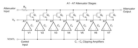
Figure 63. Simplified Voltage-Controlled Attenuator (Analog Structure)
