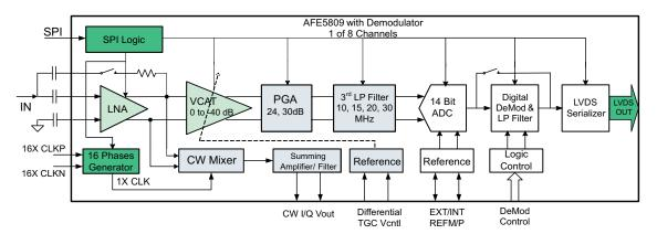
Figure 60. Simplified Functional Block Diagram
