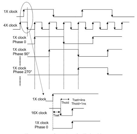
Figure 72.  $8 \times f_{cw}$  and  $4 \times f_{cw}$  Timing Diagram
