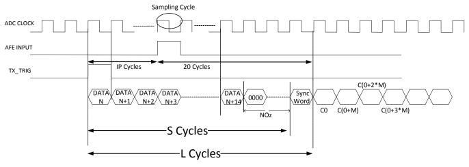
Figure 96. Measured Latency Timing at Any M
