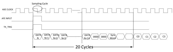
Figure 93. Expected Latency Timing When M = 1
