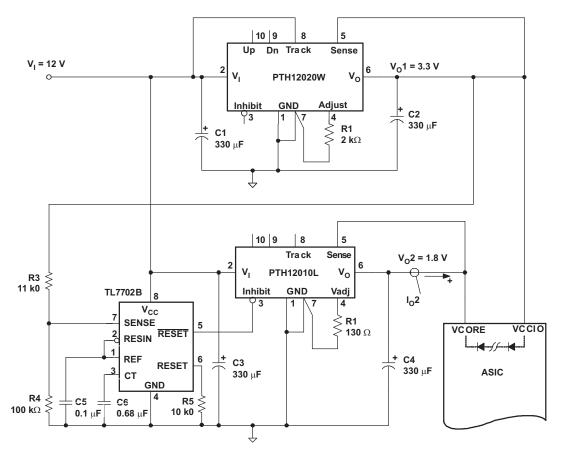
Figure 18. Application Circuit Demonstrating Prebias Startup
