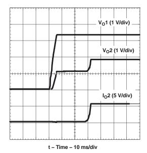
Figure 17. Prebias Startup Waveforms
