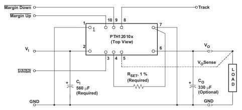
A. R<sub>SET</sub> = Required to set the output voltage to a value higher than the lowest value (see the electrical characteristics table for values).
