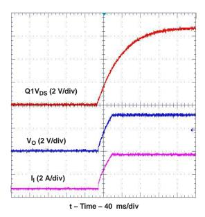
Figure 13. Power-Up from Track Control
