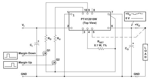
Figure 19. Margin Up/Down Application Schematic
