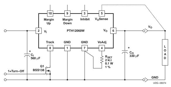
Figure 12. Basic Start-up Control Circuit
