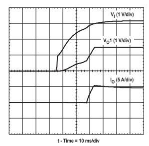
Figure 15. Prebias Start-Up Waveforms
