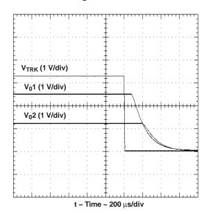
Figure 13. Simultaneous Power Down With Auto-Track Control
