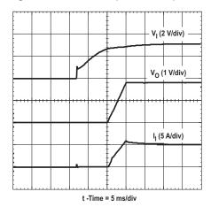
Figure 8. Power-Up Waveform
