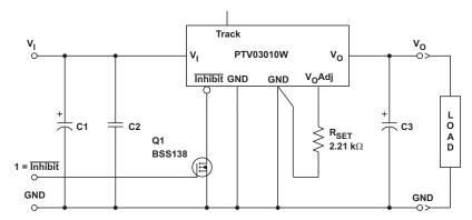
Figure 9. On/Off Inhibit Application Circuit
