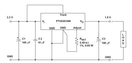
Figure 7. Power-Up Application Circuit
