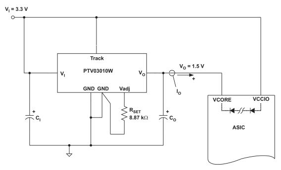
Figure 16. Application Circuit Demonstrating Prebias Start-Up
