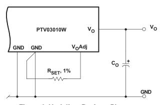
Figure 6. Vo Adjust Resistor Placement
