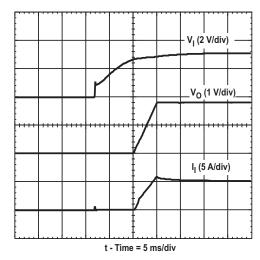
Figure 8. Power-Up Waveform
