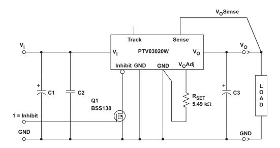
Figure 9. On/Off Inhibit Application Circuit
