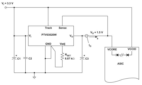
Figure 16. Application Circuit Demonstrating Prebias Start-Up
