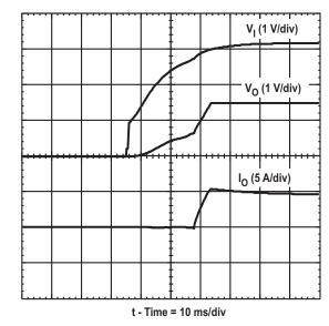
Figure 15. Prebias Start-Up Waveforms
