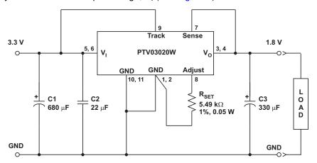
Figure 7. Power-Up Application Circuit
