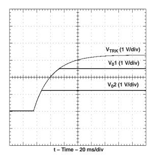
Figure 12. Simultaneous Power Up With Auto-Track Control
