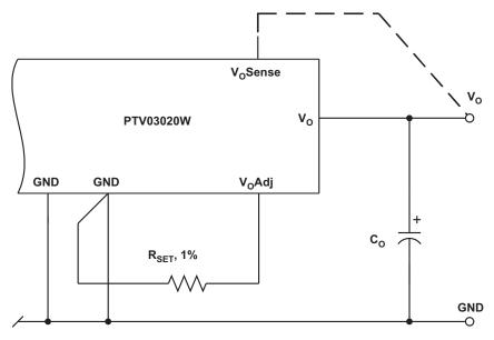
Figure 6. V<sub>O</sub> Adjust Resistor Placement
