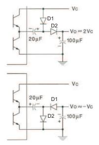
Figure 4. Charge Pump Circuit
