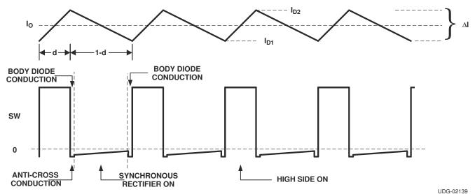
Figure 8-1. Inductor Current and SW Node Waveforms
