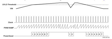
Figure 7-2. Undervoltage Lockout Operation
