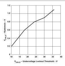
Figure 6-3. Undervoltage Lockout Threshold vs Hysteresis
