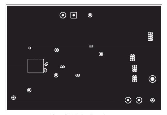
Figure 10-5. Bottom Layer Copper
