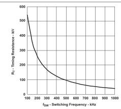
Figure 6-1. Switching Frequency vs Timing Resistance
