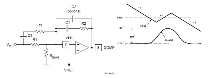
Figure 7-7. Type III Compensation Configuration Figure 7-8. Type III Compensation Gain and Phase
