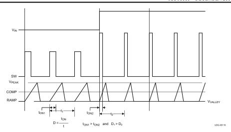
Figure 7-1. Voltage Feedforward Effect on PWM Duty Cycle
