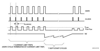
Figure 7-4. Typical Current Limit Protection Waveforms
