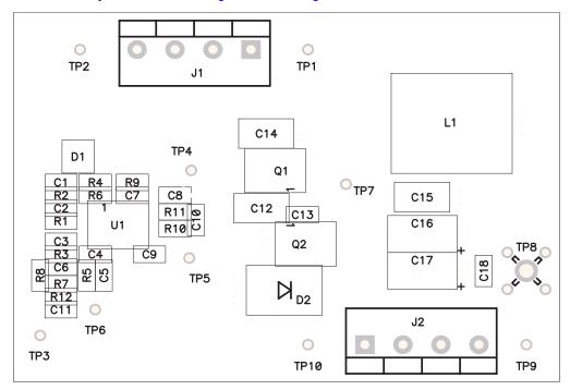
Figure 10-1. Top-Side Component Assembly
