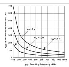
Figure 6-2. Feed-Forward Impedance vs Switching Frequency
