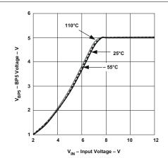
Figure 6-4. Input Voltage vs BP5 Voltage
