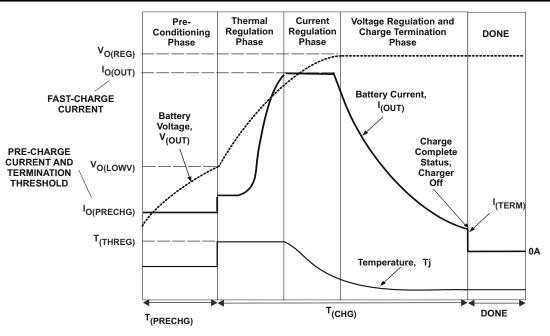
Figure 7-1. Charging Profile With Thermal Regulation
