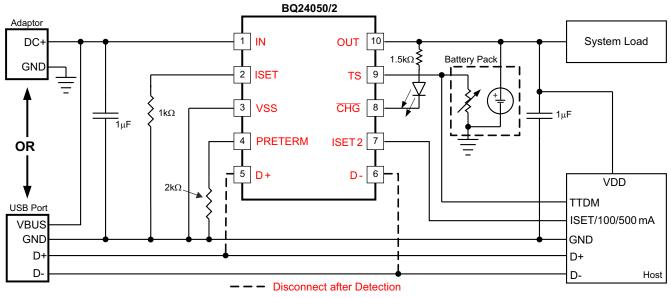
I<sub>OUT\_FAST\_CHG</sub> = 540 mA; I<sub>OUT\_PRE\_CHG</sub> = 108 mA; I<sub>OUT\_TERM</sub> = 54 mA
