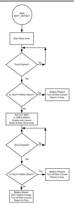
Figure 7-6. Battery Detect Flow Diagram
