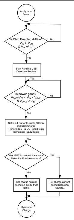
Figure 7-3. Power Up Flow Diagram
