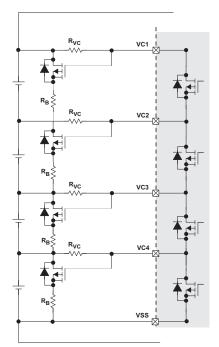
Figure 5. External Cell Balancing with  $R_B$
