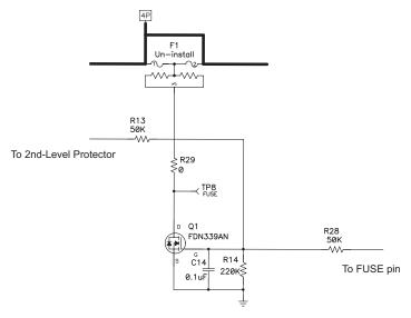
Figure 15. FUSE Circuit
