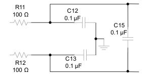
Figure 11. Differential Low-Pass Filter
