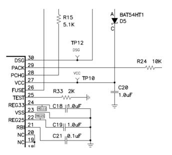
Figure 12. Power Supply Decoupling
