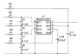
Figure 19. bq29705 Cell Inputs and Time-Delay Capacitor
