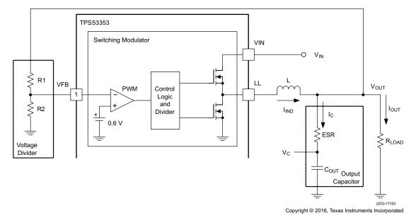
Figure 7-4. Simplified Modulator Model
