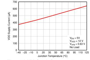
Figure 6-1. VDD Supply Current vs. Junction Temperature
