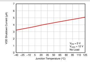
Figure 6-2. VDD Shutdown Current vs. Junction Temperature
