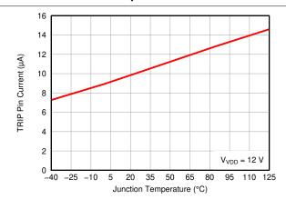
Figure 6-3. TRIP Pin Current vs. Junction Temperature
