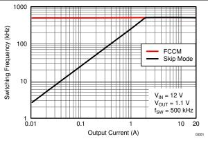
Figure 6-6. Switching Frequency vs. Output Current
