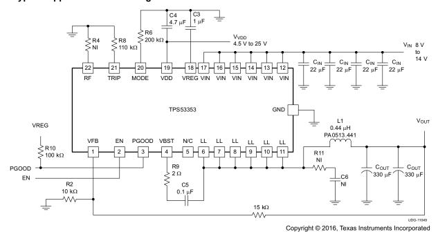
Figure 8-1. Typical Application Circuit Diagram
