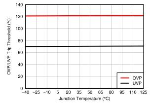
Figure 6-4. OVP/UVP Trip Threshold vs. Junction Temperature
