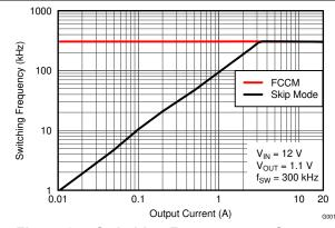
Figure 6-5. Switching Frequency vs. Output Current
