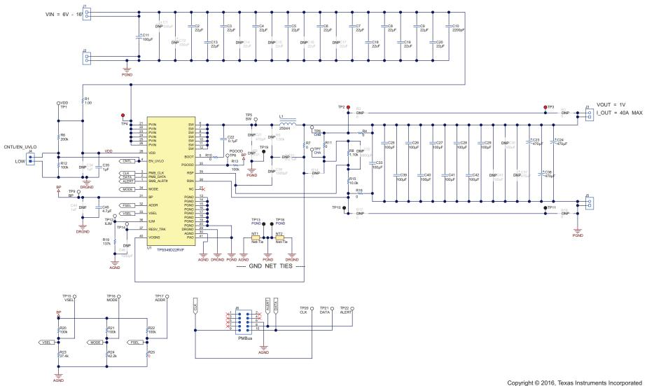
Figure 53. Typical Application Schematic
