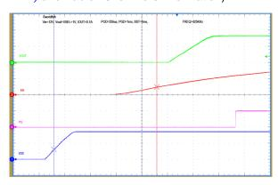
Figure 27. Proper Sequencing of V<sub>DD</sub> and EN\_UVLO to Support the Use of 4-ms SS Setting
