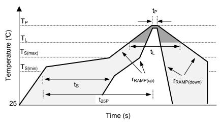
Figure 70. Recommended Reflow Oven Thermal Profile
