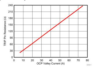
Figure 26. Current Limit Resistance vs OCP Valley Overcurrent Limit
