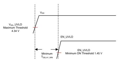
Figure 28. Minimum Delay Between  $V_{\text{DD}}$  and EN\_UVLO to Support the Use of 4-ms and 8-ms SS settings
