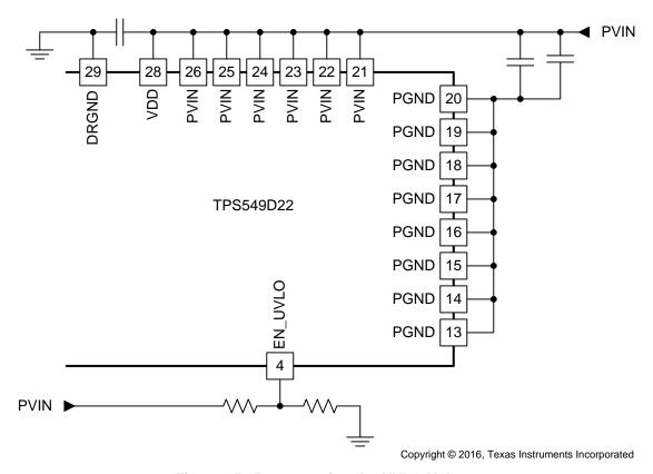
Figure 25. Programming the UVLO Voltage
