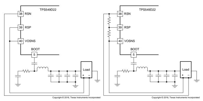
Figure 29. Remote Sensing Without Feedback Resistors
