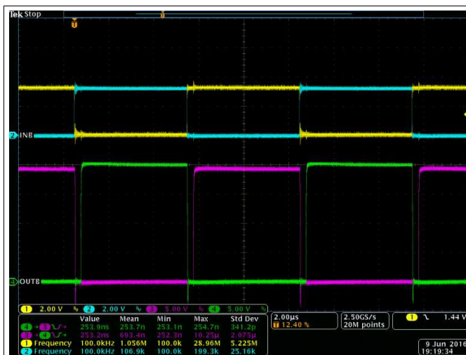
Figure 42. Bench Test Waveform for INA/B and OUTA/B
