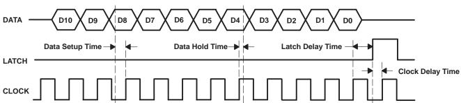
NOTE: Data is clocked in on the positive edge of the clock. The positive edge of the latch signal should occur before the next positive edge of the clock. For definition of D0 to D10, see the control logic table.
