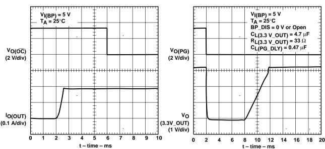
Figure 15. OC Response (BP Switch), Device Enabled Into Short
