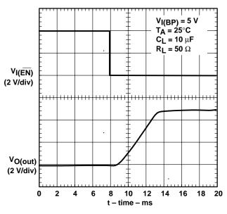
Figure 3. Turnon Delay and Rise Time (BP Switch)
