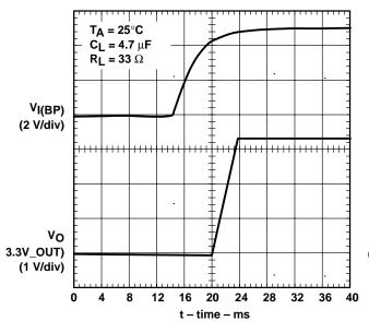
Figure 7. Turnon Delay and Rise Time (3.3V\_OUT)
