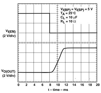
Figure 5. Turnon Delay and Rise Time (SP Switch)
