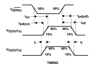
Figure 2. Timing and Internal Voltage Regulator Transition Waveforms
