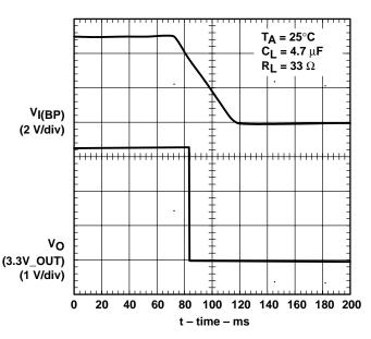
Figure 8. Turnoff Delay and Fall Time (3.3V\_OUT)
