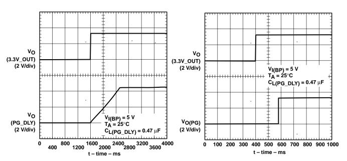
Figure 9. PG\_DLY Rise Time With a 0.47-μF Capacitor
