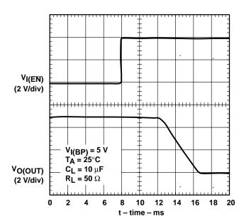
Figure 4. Turnoff Delay and Fall Time (BP Switch)
