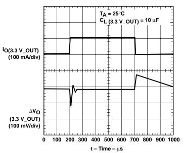
Figure 21. Load Transient Response
