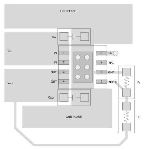
Figure 30. Recommended Layout – Adjustable-Voltage Version
