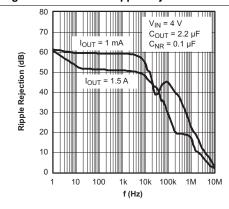
Figure 12. TPS78630 Ripple Rejection vs Frequency
