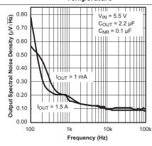
Figure 4. TPS78630 Output Spectral Noise Density vs Frequency
