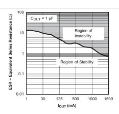
Figure 20. TPS78630 Typical Regions of Stability Equivalent Series Resistance (ESR) vs Output Current
