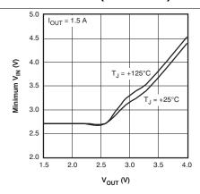
Figure 19. Minimum Required Input Voltage vs Output Voltage
