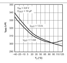
Figure 3. TPS78628 Ground Current vs Junction Temperature
