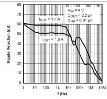
Figure 11. TPS78630 Ripple Rejection vs Frequency
