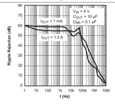
Figure 10. TPS78630 Ripple Rejection vs Frequency
