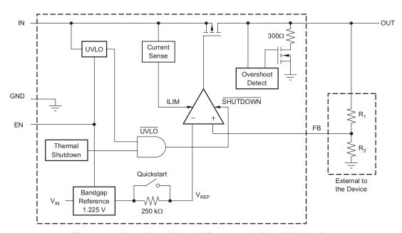
Figure 24. Functional Block Diagram—Adjustable Version
