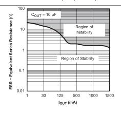
Figure 22. TPS78630 Typical Regions of Stability Equivalent Series Resistance (ESR) vs Output Current
