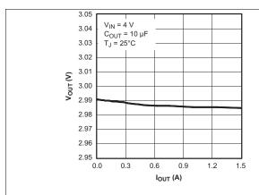
Figure 1. TPS78630 Output Voltage vs Output Current
