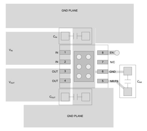
Figure 31. Recommended Layout – Fixed-Voltage Version
