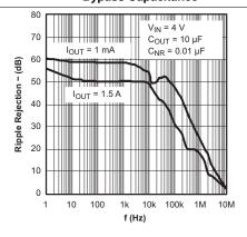
Figure 9. TPS78630 Ripple Rejection vs Frequency
