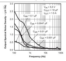
Figure 6. TPS78630 Output Spectral Noise Density vs Frequency
