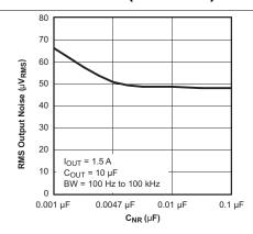
Figure 7. TPS78630 Root Mean Squared Output Noise vs Bypass Capacitance
