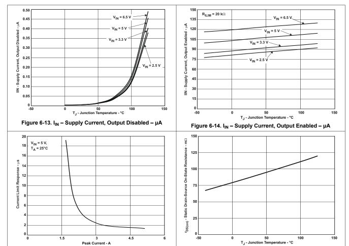
Figure 6-16. MOSFET  $r_{DS(on)}$  Vs. Junction Temperature
