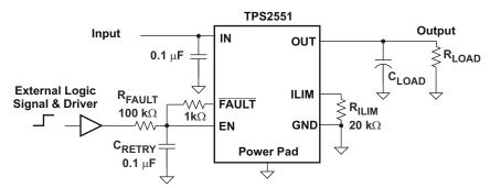
Figure 9-3. Auto-Retry Functionality With External EN Signal
