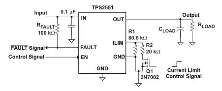
Figure 9-1. Two-Level Current-Limit Circuit
