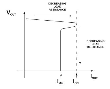
Figure 7-3. Output Voltage vs. Current-Limit Threshold
