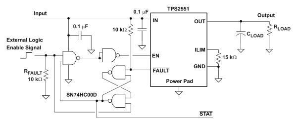
Figure 9-4. Overcurrent Latch-Off Using a Quad-NAND Gate
