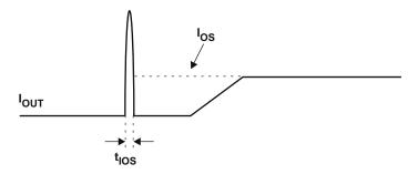
Figure 7-2. Response Time to Short-Circuit Waveform
