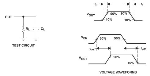
Figure 7-1. Test Circuit and Voltage Waveforms
