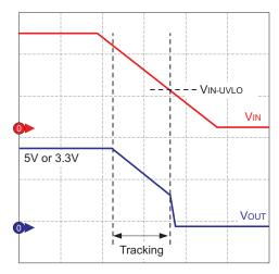
Figure 18. Undervoltage Shutdown and Low-Voltage Tracking
