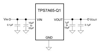
Figure 20. Typical Application Schematic
