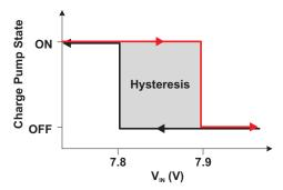
Figure 16. Charge-Pump Operation at Light Loads
