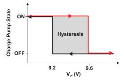
Figure 17. Charge-Pump Operation at Heavy Loads
