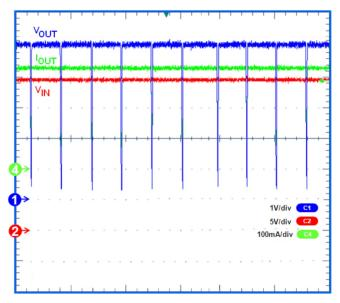
Figure 19. Thermal Cycling Waveform for TPS7A6550-Q1 ( $V_{IN}$  = 24 V,  $I_{OUT}$  = 300 mA,  $V_{OUT}$  = 5 V)
