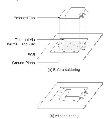
Figure 23. Using a Multilayer PCB and Thermal Vias for Adequate Heat Dissipation
