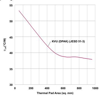
Figure 24.  $\theta_{JA}$  vs Thermal Pad Area
