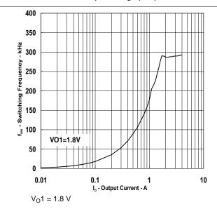
Figure 14. Switching Frequency vs
