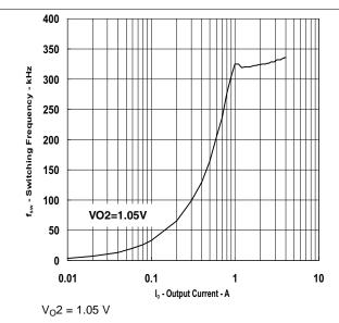
Figure 15. Switching Frequency vs
