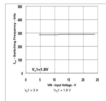
Figure 12. Switching Frequency vs
