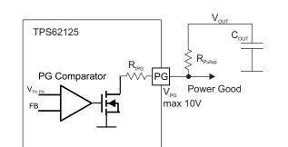
Figure 11. PG Open Collector Output
