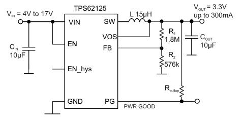
Figure 8. TPS62125 3.3-V Output Voltage Configuration
