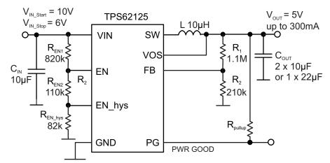
Figure 58. TPS62125 5-V V<sub>OUT</sub>, Start-up Voltage V<sub>IN\_Start</sub> = 10 V, Stop Voltage V<sub>IN\_Stop</sub> = 6 V, See Figure 47
