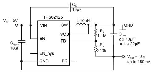
Figure 60. 5 V to -5 V Inverter Configuration, See SLVA514
