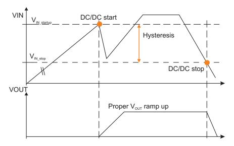
Figure 10. Using the EN Comparator as Input SVS for Proper V<sub>OUT</sub> Ramp Up
