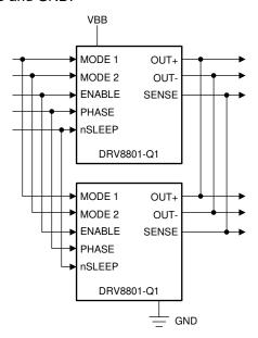
Figure 8-6. Functional Block Diagram (Connected Signals)
