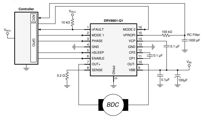
Figure 8-1. Typical Application Schematic
