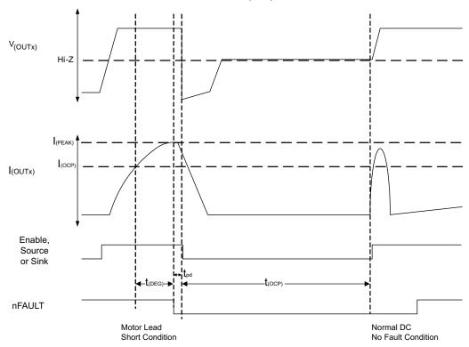
Figure 7-2. Overcurrent Control Timing
