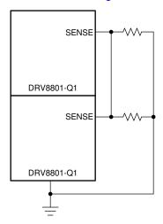
Figure 8-10. SENSE Resistors Connection
