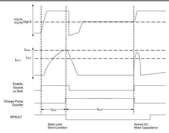
Figure 6-2. Overcurrent Control Timing
