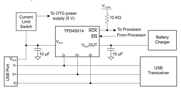
Figure 16. OTG Schematic
