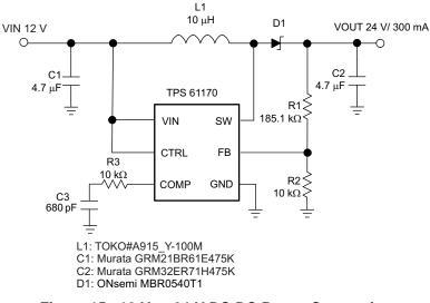
Figure 15. 12-V to 24-V DC-DC Power Conversion
