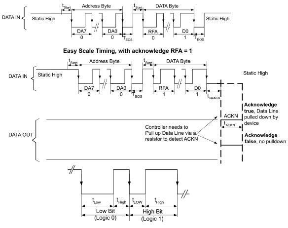
Figure 13. EasyScale — Bit Coding
