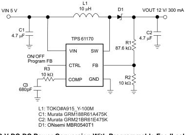
Figure 18. 5-V to 12-V DC-DC Power Conversion With Programmable Feedback Reference Voltage
