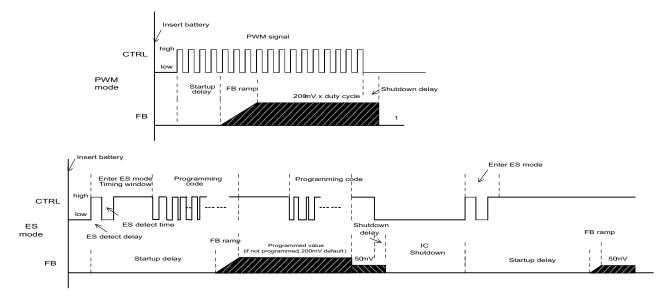
Figure 14. Mode Detection of Feedback Reference Program
