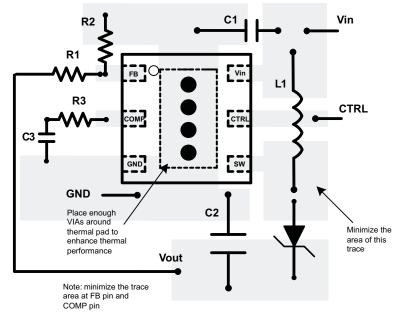
Figure 20. PCB Layout Recommendation
