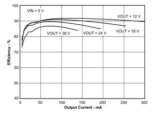
Figure 17. Efficiency vs Output Current
