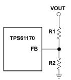
Figure 16. Program Output Voltage
